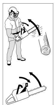
If the kickback is less violent or the kickback zone of the bar is closer to you the chain brake will be activated manually by the movement of your left hand
